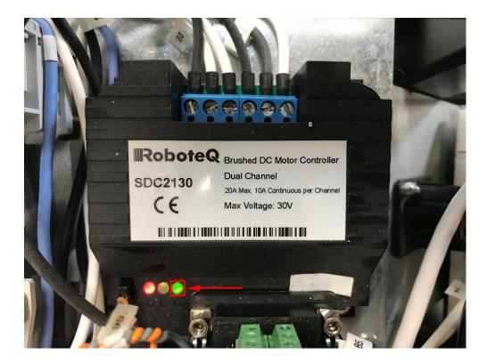
Figure 1.4. Motor controller LED
