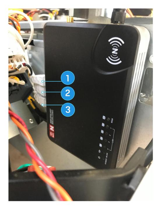
Figure 1.3. Router and its inputs
